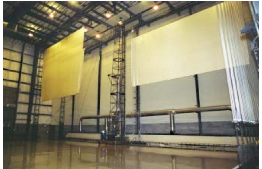
Screen coating plant at Harkness Hall's Fredericksburg USA facility. The spray tower is centre left.
